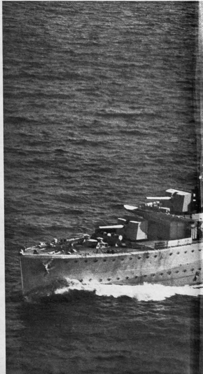
"A" AND "B" CLASS ships like Antelope (below) were first to mount their torpedo tubes in banks of four, to introduce box-shaped shields.
